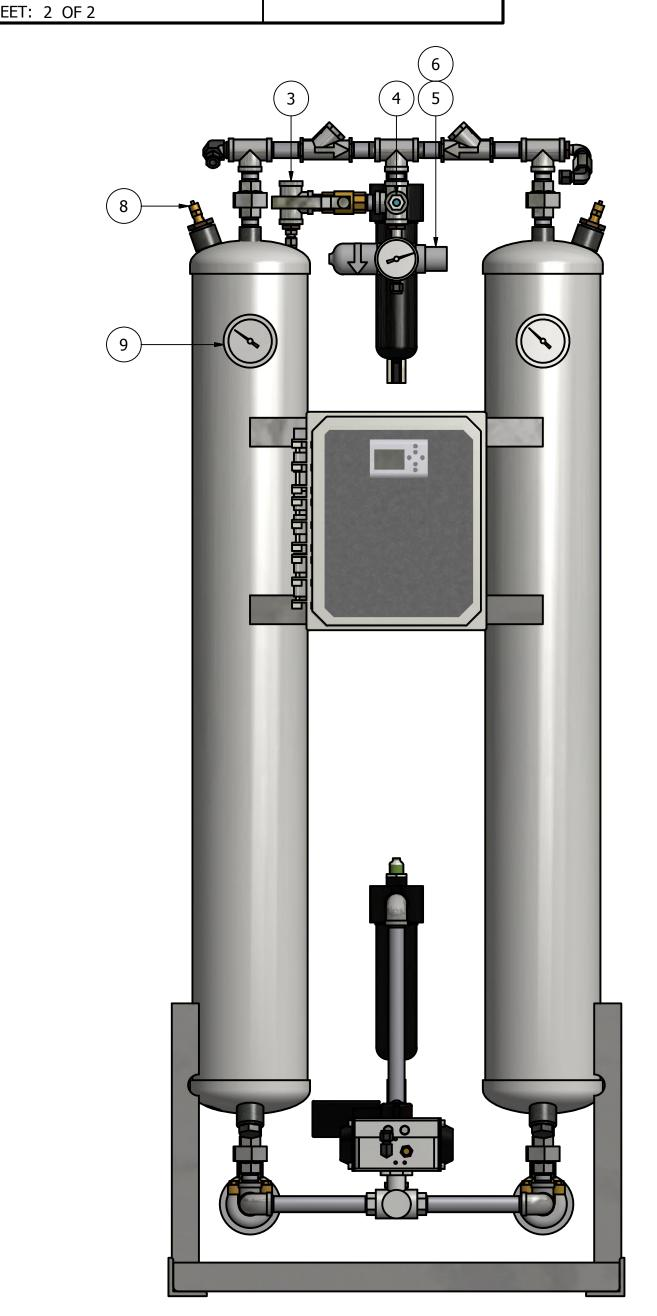
PARTS LIST QTY DESCRIPTION **ITEM** CHECK VALVE, OUTLET 2 PARTICULATE AFTER-FILTER 2 1 DEW POINT MONITOR (OPTIONAL) 3 1 MOISTURE INDICATOR 1 4 PRESSURE REGULATOR, CONTROL 5 1 PRESSURE GAUGE, CONTROL 6 1 NEEDLE VALVE, PURGE 7 1 RELIEF VALVE, TANK 8 2 PRESSURE GAUGE, TANK 9 2 10 3 WAY BALL VALVE, INLET COALESCER PRE-FILTER 11 1 TIMED DRAIN 12 1 SOLENOID, EXHAUST 2 13 MUFFLER, EXHAUST 2 14 55 LBS DESICCANT
